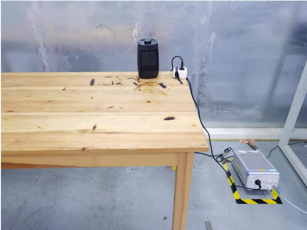
Photo of Power Line Conducted Measurement
