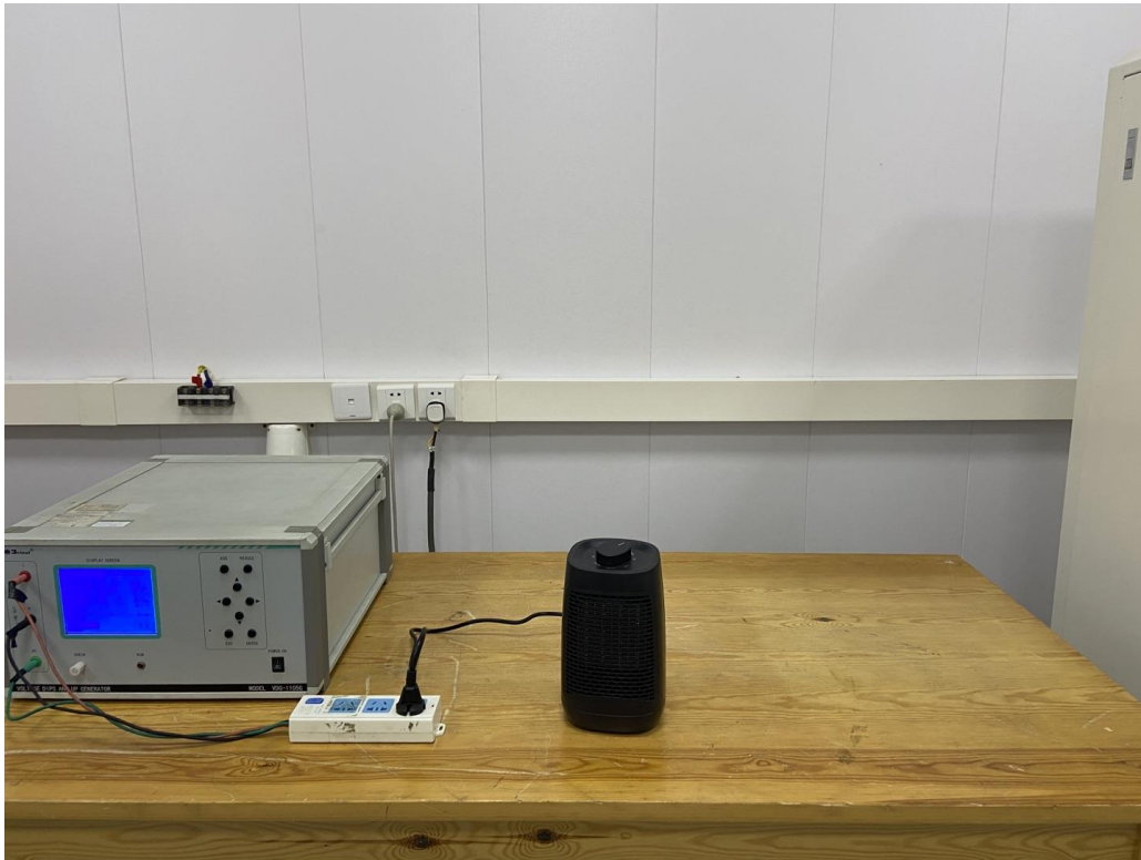
Photo of Voltage Dips and Interruptions Test
