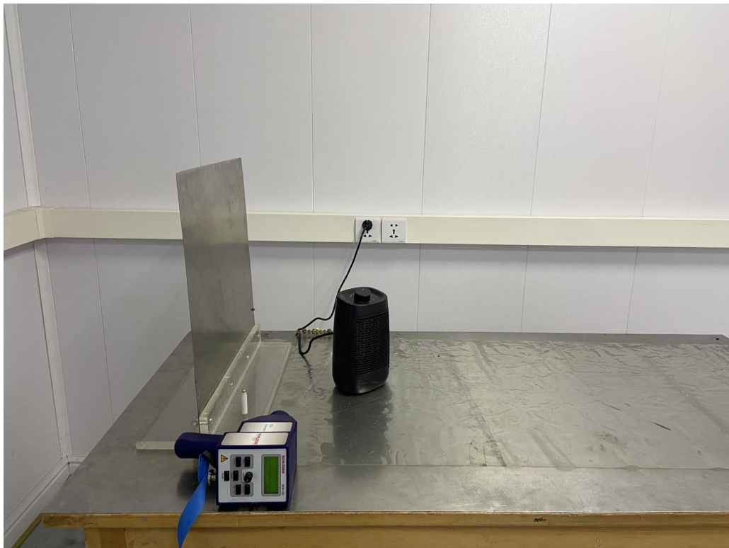
Photo of Electrostatic Discharge Test
