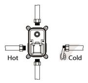
Depth of the outlet pipe: pipe bracket is installed 0.2 inch (5mm) from the front of the finished wall (as picture below)
