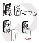
2) During the test, open the water supply system, flush the two outlet pipes by operating the handle, and test whether the water pressure is appropriate.
