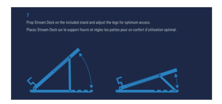
Prop Stream Deck on the included stand and adjust the legs for optimum access.
