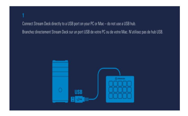
Connect Stream Deck directly to a USB port on your PC or Mac – do not use a USB hub.
