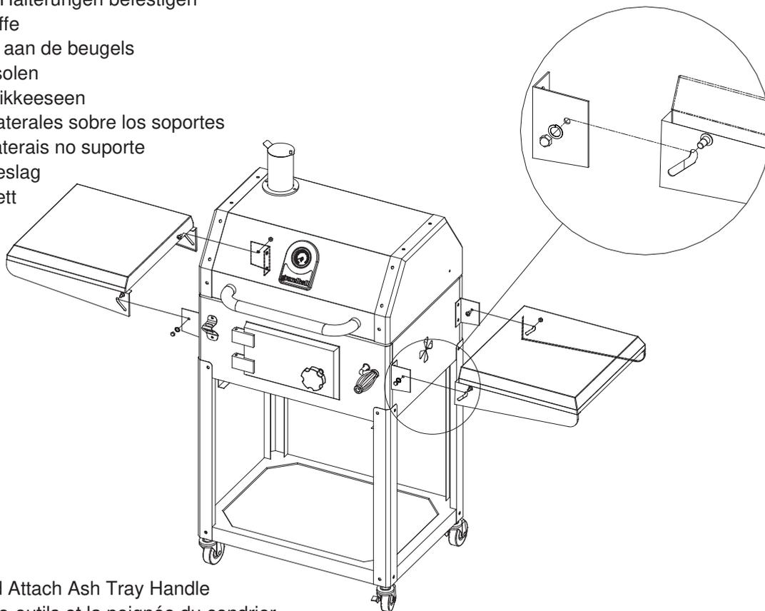
19. (GB) Attach Tool Hooks and Attach Ash Tray Handle
