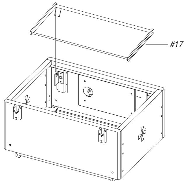
9. (GB) Attach charcoal tray wire and place it on the charcoal tray lifting bracket
