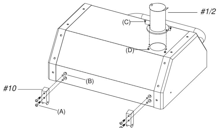
3. (GB) Attach Crank Bracket To Front Panel
