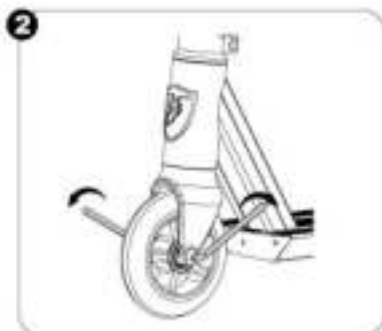
Securely tighten the bolt as shown.
