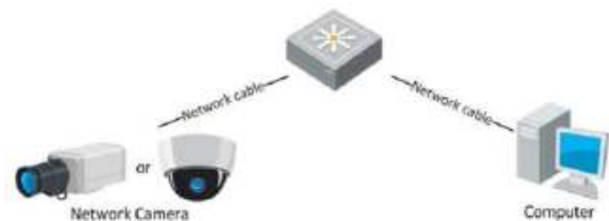
Figure 2-2 Connecting via a Switch or a Router
