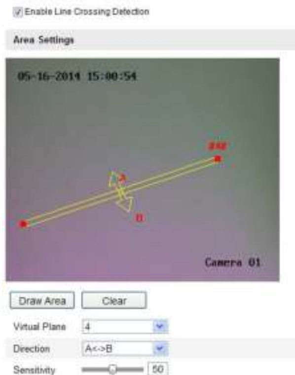
Figure 6-60 Draw Crossing Line
