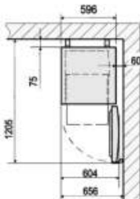
The heated air around the rear of the unit must be able to circulate freely. Therefore, ensure that the air circulation behind the unit is not obstructed.
