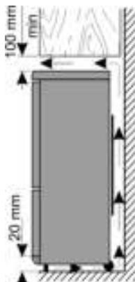
If the refrigerator is installed with its side against a wall, ensure a minimum clearance of 60 mm to ensure that the door can open through 90°.
