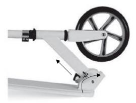
Make sure to fully unfold until you hear the "snap in". Close the quick release. Make sure it's tight.
