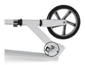
By pulling the trigger, you can unfold the scooter.
