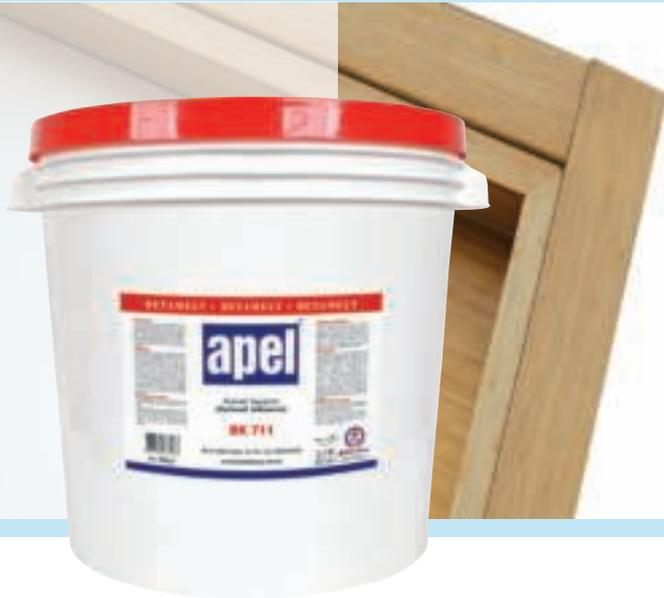
Apel BK 711 is an EVA based granule hotmelt glue, produced of high quality synthetic resins which is used for bonding solid MDF materials in door frame production industry. The glue has a low/mid viscosity values, good surface wetting ability and high thermal resistance. It is mostly used for bonding MDF pieces in automatic door jamb bonding machines in high temperatures. For an optimum bonding quality, the machine speed is suggested to be 15 m/min.
