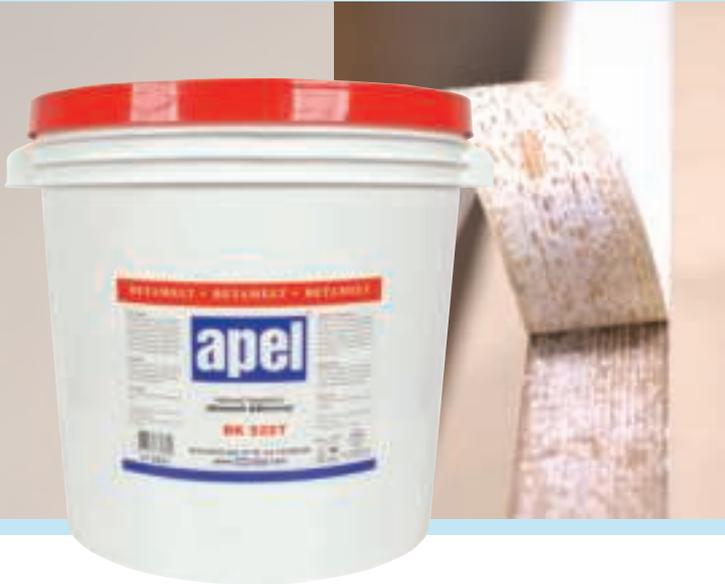
Apel BK 522T is a hotmelt glue for automatic straight edgebanding machines especially designed for slot nozzle glue applications. With its low viscosity, it has a high wetting ability. It is an EVA based hotmelt granule shaped glue that melts in high temperatures.
