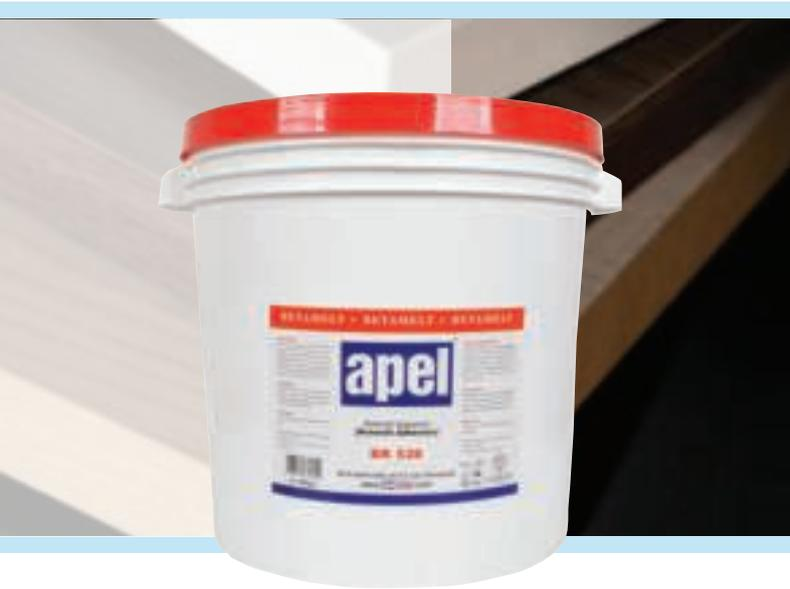
Apel BK 528 is a natural colored edge-banding glue with medium open time and excellent final bonding. It is specially formulated for medium speed (12 - 18 m/min), roller-press, automatic straight edge-banding machines. It can be used to bond wood, PVC, melamine, ABS edge-bands to MDF, chipboard or solid wood boards. Not suitable for acrylic edge-bands.
