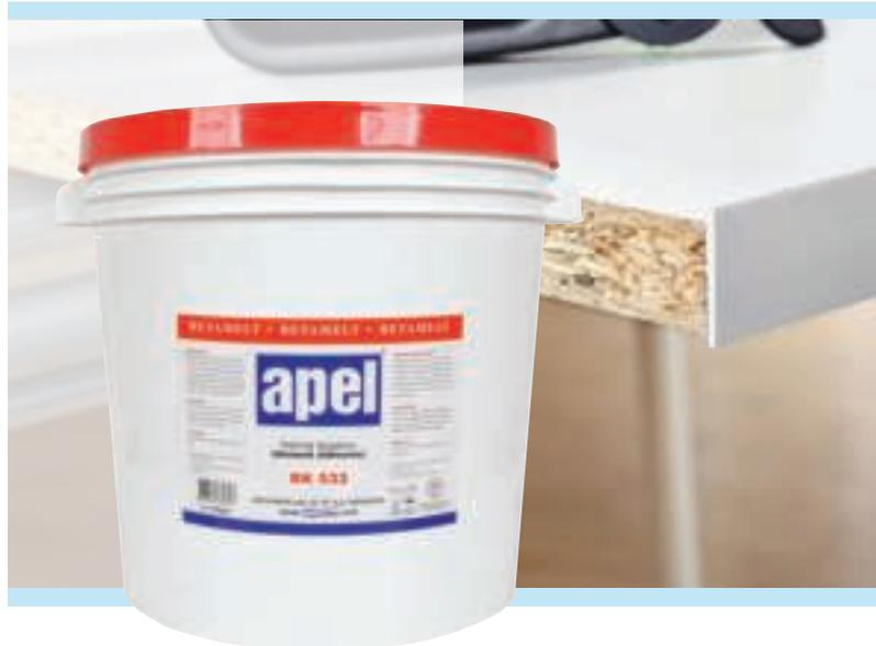
Apel BK 533 is a semi-natural colored edge-banding glue with long open time and excellent final bonding. It is specially formulated for low and medium speed (8 - 15 m/min) automatic edge-banding machines. It can be used to bond wood, PVC, melamine, ABS edge-bands to MDF, chipboard or solid wood boards. Not suitable for acrylic edge-bands.
