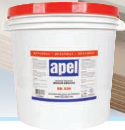
Apel BK 538 is a semi-natural colored edge-banding glue with long open time and excellent final bonding. It is specially formulated for low and medium speed (8 - 12 m/min) automatic edge-banding machines. It can be used to bond wood, PVC, melamine, ABS edge-bands to MDF, chipboard or solid wood boards. Not suitable for acrylic edge-bands. Good price/performance ratio.
