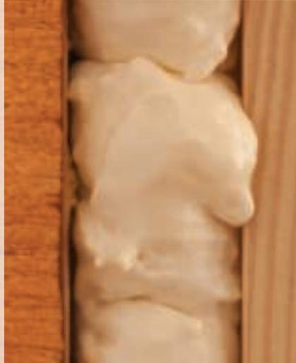
APEL PF 340 is a polyurethane foam cured with the moisture in the atmosphere and the substrate surfaces. Due to its special formulation, the foam can be used in harsh and cold weather conditions.
