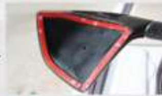
② Attach double-sided tape
