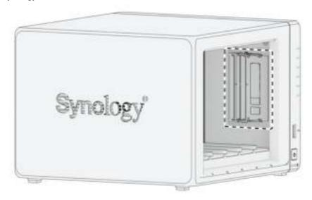
**Note:** When you remove the drive trays, sensitive internal components are exposed. Avoid touching anything other than the memory assembly when removing or adding memory.
