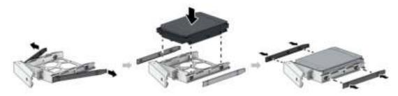
• For 2.5" drives: Remove the fastening panels from the sides of the drive tray and store them in a safe place. Place the drive in the area of the drive tray indicated below. Turn the tray upside down and tighten the screws to secure the drive in place.
