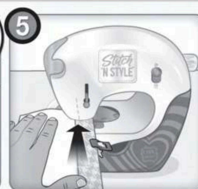
Guide fabric with hand and let the Presser Foot automatically push the fabric forward. IMPORTANT: Do not push or pull the fabric while sewing. TIP: Use the PLAY/PAUSE switch to START and STOP while sewing.
