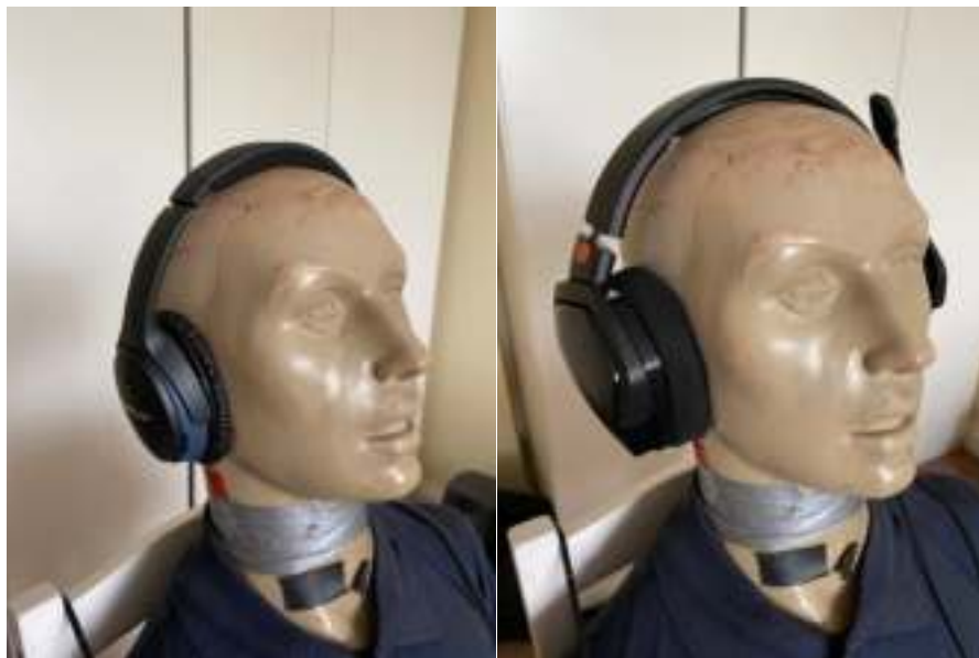
Figure 2: Typical fit of BOSE (left) and N16 (right) headphones on HATS
