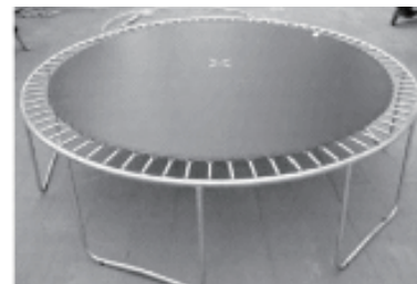
13. Secure all remaining springs. Always two opposing springs one after the other.
