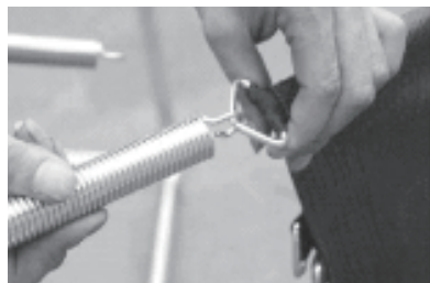
9. After all the springs are inserted into the frame, insert the bounce mat into the frame. Attach a spring onto a hook on the bounce mat.
