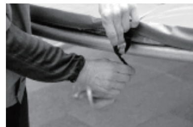
15. Attach the frame cover with black bands to the frame or the support legs. Do not attach them to the springs.
