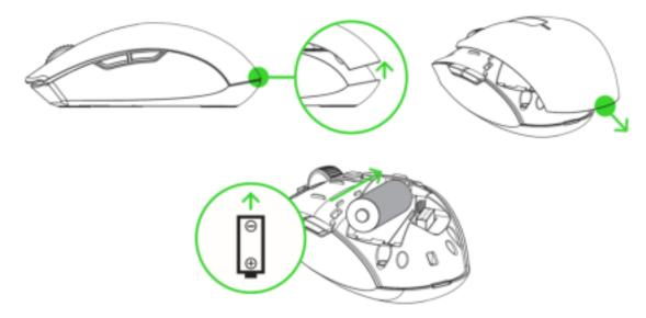
Caution: The included AA battery is non-rechargeable. You may also use a AAA battery (not included) if preferred. Do not simultaneously use AA and AAA batteries; only one (1) battery is required to use the mouse. Dispose batteries in accordance with your local environmental laws. For your safety, use only lithium or alkaline batteries.
