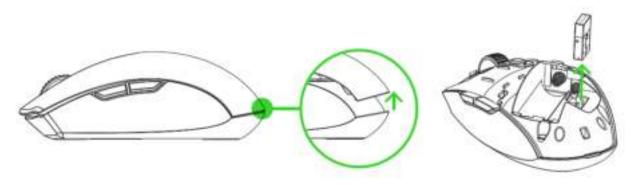
2. Close the top cover and insert the wireless USB dongle into the USB port of your PC.
