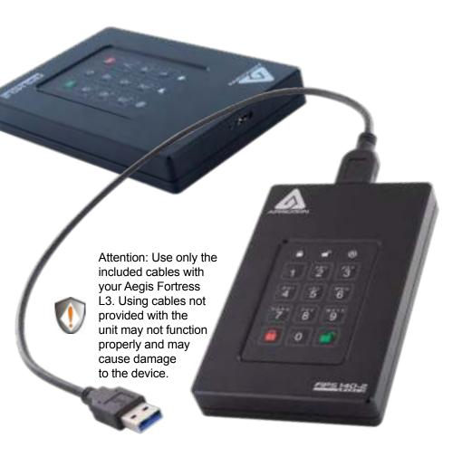
When you first plug in the Fortress L3, the unit will do a self-test to verify all security components are working properly. The LEDs will go through 3 test stages **RED**, **GREEN**, and **BLUE**. This will be followed by three **GREEN** flashes on a successful test. Any test failure will leave the unit in an inoperable state indicated by a flashing **RED** LED. Should this occur, contact our Tech Support department.
