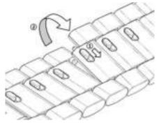
**2** To install a strap, push the lever in the direction indicated by arrow 1 and then install the chain in the direction indicated by arrow 2.
