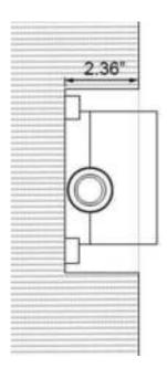
(3) Connecting the inlet and outlet pipe with the valve body; Please notice that before connecting the shower control valve, flush the water inlet pipe to ensure the water in let pipe has no impurities;
