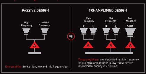
Unlike most conventional soundbars that utilize a single amplifier to reproduce the entire audio spectrum, Sound BlasterX Katana employs three high-performance amplifiers – one dedicated to driving lows, one for mids, and another solely for high frequencies.
