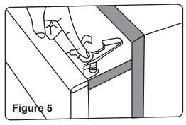
Improvement: It's no need to take off the safety lock when it's done using. The lever could hold the lock down and there is no need to press the spring everytime when opening the cabinet, drawer, or door. It could be always ready for the second use and causes no damage to the furnitures.
