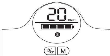
2. When the scooter is switched on, double-click quickly to shift gears (2 gears in total).
