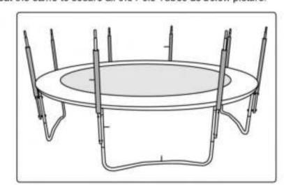
Place the upper pole B in the pockets of the safety net.
