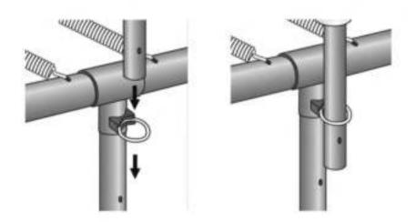
STEP 2: Align holes, secure the poles with Long Bolt (5), Plastic Spacer (3), Washer (4) and Dome Nut (6).
