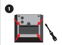
SCREW OFF THE COVER OF THE BATTERY COMPARTMENT
