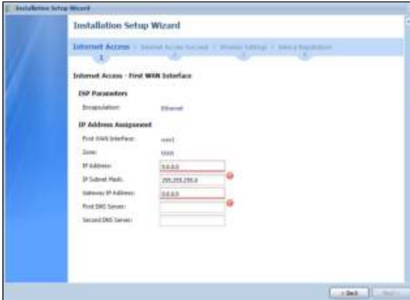
Figure 24 Internet Access: Ethernet Encapsulation
