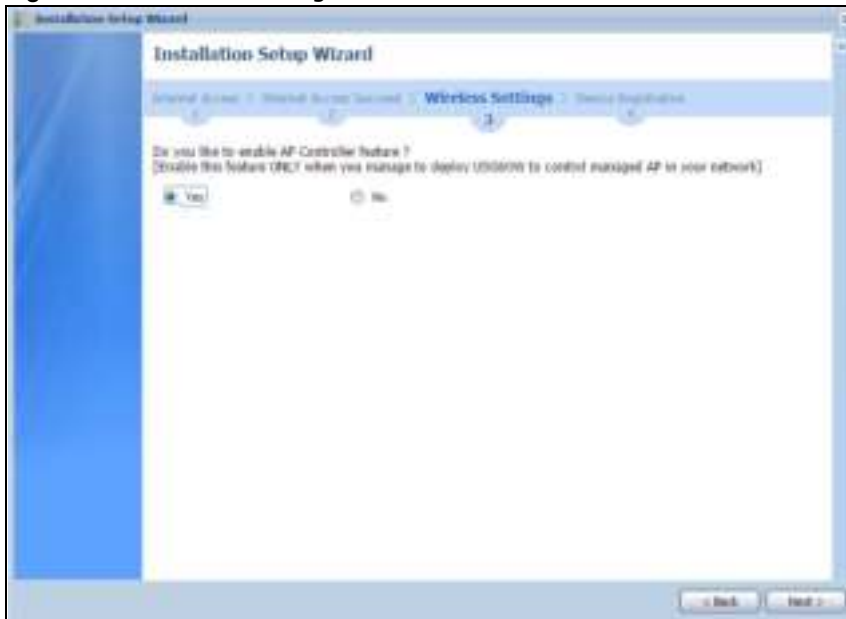
Figure 29 Wireless Settings: AP Controller
