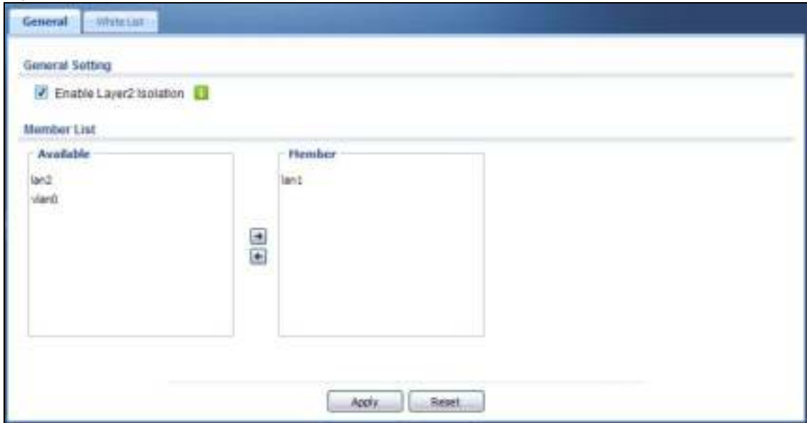
Figure 227 Configuration > Network > Layer 2 Isolation
