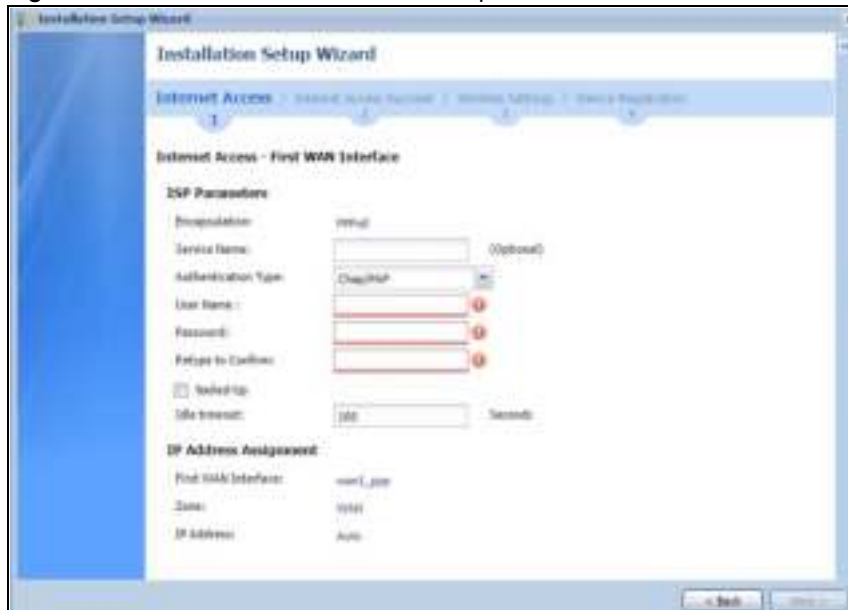
Figure 25 Internet Access: PPPoE Encapsulation
