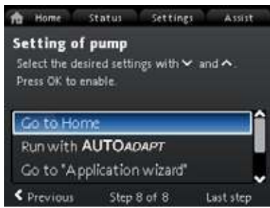
Fig. 57 Startup guide: Setting of the pump
