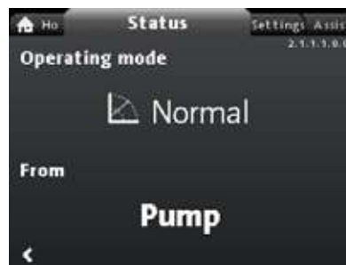
Fig. 58 Example of the submenu "Operating status" showing the pump running in normal operation in a multipump system.
