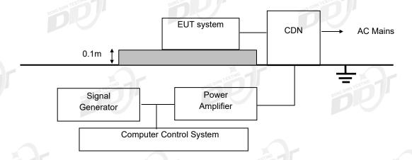
For audio output function (electrical measurement, direct connection to EUT)
