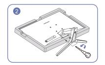
Remove the screws from the bottom of the stand neck.
