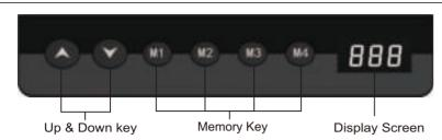
The whole handset surface is a button panel. If there is no press within 30 seconds, the screen is locked and M1/M2/M3/M4 keys are locked correspondingly, you should press Up or Down key first, it can be used when the display screen light up.
