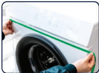
5. Adjust the height of all the feet. Make sure they are on an equal level according to the horizontal meter
