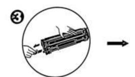
Pull out the sealing tape slowly with horizontal force to avoid breaking of sealing tape.
