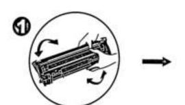
When produced, toner is housed inside the toner hopper. Before usage, shake the toner hopper 6-8 times to make sure the toner is loose and evenly distributed inside.
