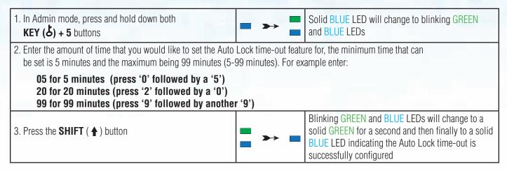
**Note:** To immediately exit Admin Mode (solid BLUE LED), press and hold down the **SHIFT** (♠) button for a second - the solid BLUE LED switches to a solid RED LED.
