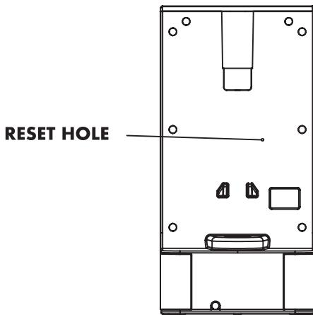
The appliance have manual thermostat to recover the heating function for abnormal operation, if the unit is no power, stop working, not boiling the water, you can reset the thermostat by using the reset key to press the reset hole on the back of appliance.
