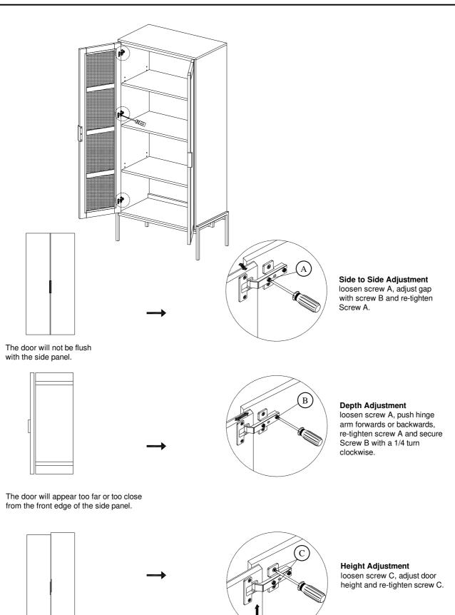
The door will not be flush with the vertical panel.
