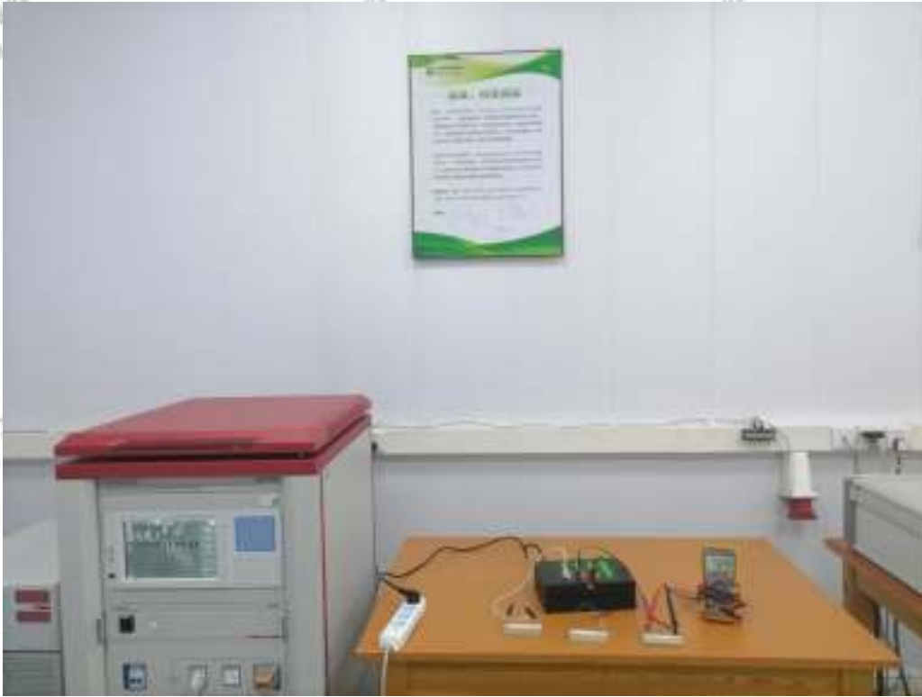
Test Setup Photo of Harmonic & Flicker Measurement
