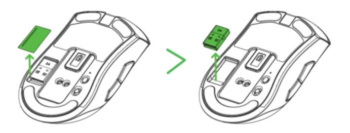
2. Reattach the compartment cover and insert the wireless USB dongle into the USB port of your PC.
