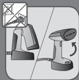
**EN** Always unfold the steam head until it is locked before any use of the appliance.
