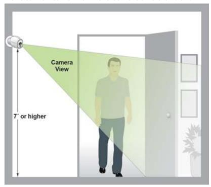
• Aim with the cloud. Use Arlo's Position mode to send video to the cloud as quickly as possible. This allows you to aim the camera while watching the video
