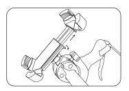
3. Release the lock lever at the back of bracket to expand the holder.
