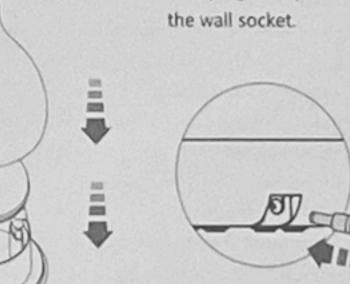
6. Plug the head of power adaptor into the power jack on the back of base
