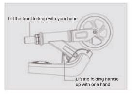
Lift the folding handle up with one hand and lift the front fork tube with another hand, an hear a "click"
