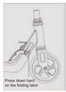
Press the folding lock firmly (the folding lock can adjust the tightness)
