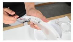
2, assemble the tubes to the petals, each petal has two tubes, the wire of the petal goes through one of the tube
