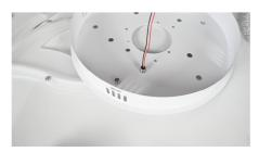
3, assemble each petal with tubes to the plate as shown, the wire goes through the inner holes of the plate
