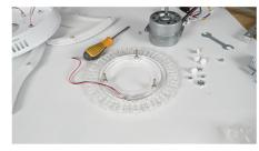
6, assemble the three bolts to the bottom plate as shown
