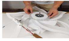
8, assemble the bottom plate to the light, find the three holes to fit the bolts and fasten with nuts
