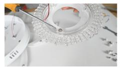
4, take off the screw from the bottom plate as shown
