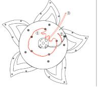
10, with series conecting way, connect the wires of all the petals together with the motor
