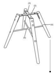
After leg completely assembled, please be sure to put the leg on the flat floor or glass platform to check if the leg is assembled well of not. If only 2 pcs of le touched the floor, please according to the photo showed and use your hand to adjust the leg which touched the floor and to make sure 4 pcs legs at the same level
