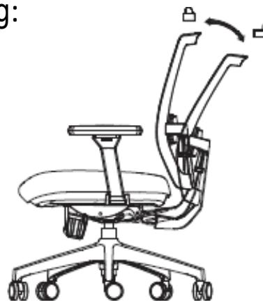
Eng. The handle (2) at the left side can also control the tilting. Pull the handle out to unlock, push it in to lock. The backrest can be locked in 3 positions.
