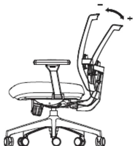
Eng. By turning the big knob (3) you can adjust the tension of the backrest when it is not locked in a fixed position.
