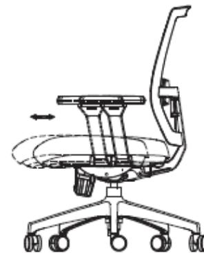
Eng. Press the level (5) and pull the seat to slide forward and backward
