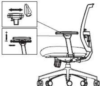
Eng. 4D armrest: armrest height adjustable, arm Pad forward / backward adjustable, arm pad pivot angel adjustable and width adjustable.
