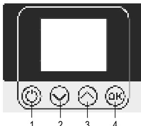
1 – Switching the convector heater On / Off;
