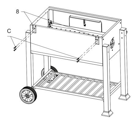
10. Lower hingers (8) are fixed to the back panel (9) with 4pcs M6\*40 screws (C).
