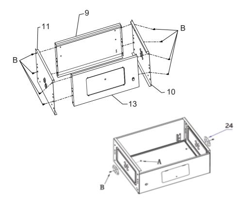
Fix side panels LH\*RH (10, 11) with 8pcs M6x12 screws (B) to front panel (13) and rear panel (9).
