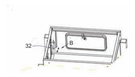
7. Handle grip (32) is fixed to the front panel (13) with 2 pcs M6\*12 screws (B).
