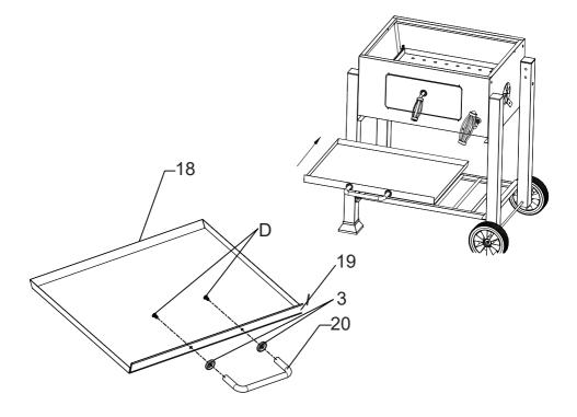
9. Fix Ash tray handle (20) and 2pcs washers (3) to Decorating strip (19) and ash tray (18) by 2pcs M6\*16 screws (D). Then fix the ash tray to the body.
