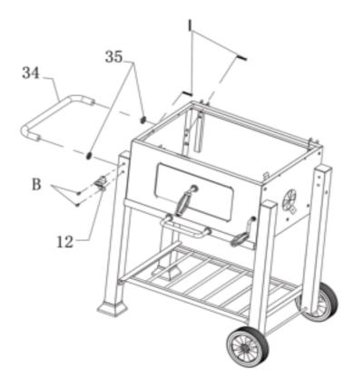
11. Bottle opener (12) is fixed on the left front leg with 2 pcs M6\*12 screws (B). Fix side handle (34) and side handle washer (35) with 2 pcs M6\*70 screws (I).
