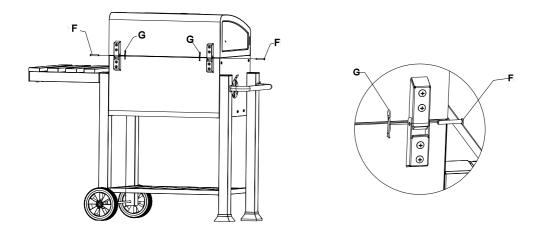
15. Lid is fixed to the body by locking the upper and bottom hinges by 2pcs pins (F) and 2pcs R clips (G).
