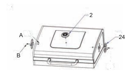
14. Fix the 2pcs air vents (24) to the lid by 2 pcs M6\*12 screws (B) and 2pcs M6 nuts (A).Fix the thermalmeter (2) on the top of lid by its own nut.
