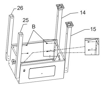
3. Fix two legs (14 & 15) with 4pcs M6x12 screws (B) to the left side panel.
