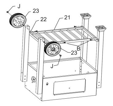
4. Fix bottom shelf (21) to the legs with 4pcs M6x12 screws (B).Fix the wheel axle (22) into the legs (25&26).Then fix the 2 wheels (23) by 2pcs M10 nuts (J).
