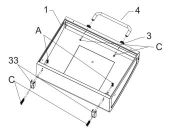
13. Fix handle for lid (4), handle washer (3) to lid (1) by 2pcs M6\*40 screws (C).
