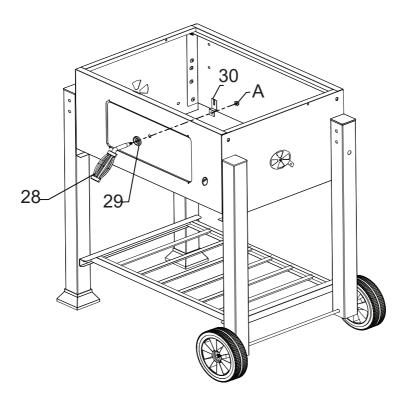
5. Fix the charcoal door handle (28), the charcoal door handle washer (29) and charcoal door locking part (30) to the front panel by 1pc M6 nut (A).
