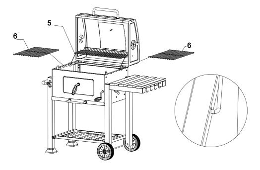
16. Fix the warming grid (5) into the lid and body. See detailed for fixing into the body.
