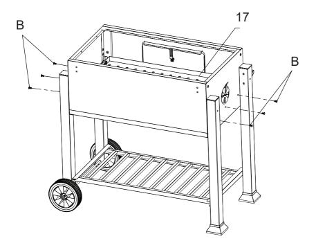
6. Charcoal pan (17) is fixed into the body with 6pcs M6\*12 screws (B).
