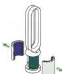
Unplug the appliance from the main electricity supply. Slide the buttons down on either side of the shrouds.
