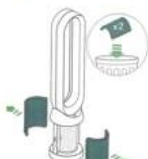
To remove the carbon filters pull the tabs on both sides of the filters. Dispose of the carbon filters in the bin.
