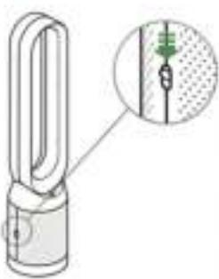
Important: Always unplug the appliance before changing filters. When the appliance detects that the non-washable glass HEPA filters need replacing the display on the appliance will show a solid purple bar.
