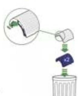
Empty the glass HEPA filters directly into the bin by pushing in both the purple tabs on the shrouds.
