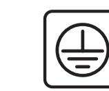
**GB** Protection class 1: the fitting must be earthed.
