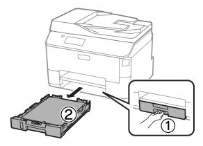
Carefully remove any paper jammed inside the printer.
