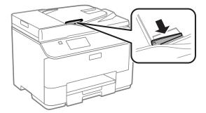
Insert the originals face-up and short edge first into the Automatic Document Feeder.
