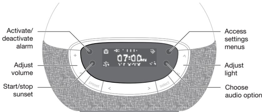
The four black buttons perform specific functions indicated by the icon next to them on the display. The bottom right icon indicates which audio option is in use.
