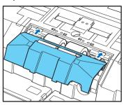
8. Push the front of the retard roller cover in. Make sure to hear a latching sound that it is securely returned to its original position.
