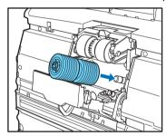
7. Put the feed roller in place (1), and align the notch in the roller's axle with the shaft on the scanner (2).
