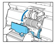
3. Pull the roller lock lever down.
