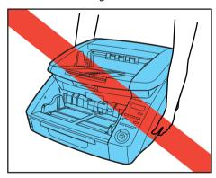
Make sure to disconnect the interface cable and power cord when moving the scanner. If the scanner is carried with these items connected, the plugs and connectors may be damaged or cause the scanner to fall and result in personal injury or damage to the scanner.
