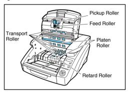
6. Remove the pickup roller, feed roller, retard roller, and retard roller cover. (See "Removing and Reinstalling the Rollers" on p. 5-9.)
